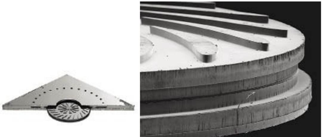
*A cross section of the microturbine (left created at the University of Maryland reveals the location of the micro ball bearings, which are contained in a notch in the edge of the turbine below the rotors (right). photos courtesy Ghodssi, McCarthy, Waits, Beyaz, Hanrahan, University of Maryland.*
